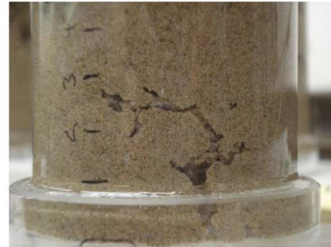
FIGURE 1 Network of channels due to stygofauna burrowing observed at the bottom of a sediment column 5 months after start of the experiments
